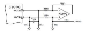
Figure 24. Single-Supply DC Differential Coupled Circuit
