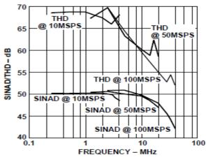
Figure 7. SINAD/THD vs. fOUT (Differential Output, AVDD and DVDD = 3.0 V)
