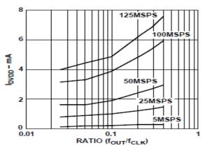
Figure 20. IDVDD vs. Ratio @ DVDD = 3 V
