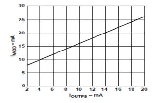
Figure 18. I<sub>AVDD</sub> vs. I<sub>OUTFS</sub>
