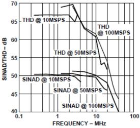
Figure 6. SINAD/THD vs. fOUT (AVDD and DVDD = 3.0 V)
