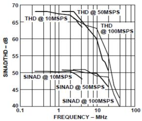
Figure 3. SINAD/THD vs.  $f_{OUT}$  (AVDD and DVDD = 5.0 V)
