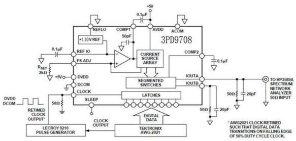
Figure 2. Basic AC Characterization Test Setup
