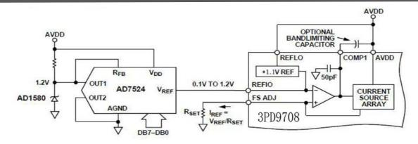
Figure 14. Single-Supply Gain Control Circuit
