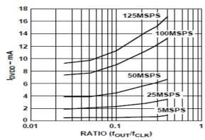
Figure 19. IDVDD vs. Ratio@ DVDD = 5 V
