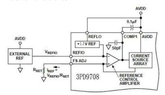
Figure 13. External Reference Configuration
