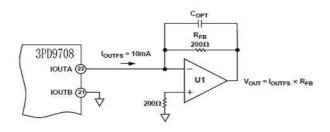
Figure 16. Unipolar Buffered Voltage Output
