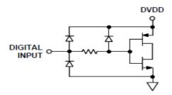
Figure 17. Equivalent Digital Input
