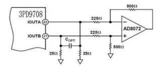
Figure 23. DC Differential Coupling Using an Op Amp
