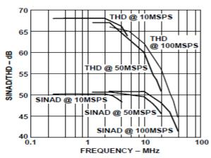
Figure 4. SINAD/THD vs. f<sub>OUT</sub> (Differential Output, AVDD and DVDD = 5.0 V)
