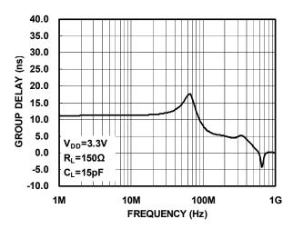
Figure 7. Group Delay vs Frequency
