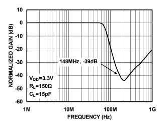
Figure8. Stop Band Attenuation
