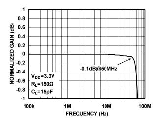
Figure 3. Small-Scale Frequency Response
