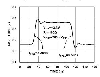
Figure 12. Small-Signal Pulse Response Vs. Time
