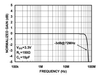
Figure 4. Large-Scale Frequency Response
