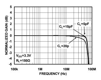
Figure 5. Gain Vs. Frequency With CLOAD
