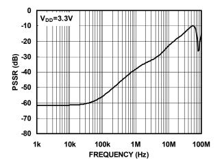
Figure 9. PSRR Vs. Frequency
