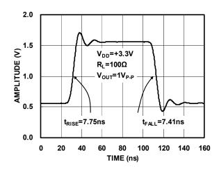
Figure 11. Large-Signal Pulse Response Vs. Time
