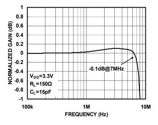
Figure1. Small-Scale Frequency Response
