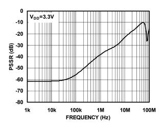
Figure8. PSRR Vs. Frequency(FHD)
