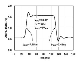
Figure11. Large-Signal Pulse Response Vs. Time(FHD Channel)
