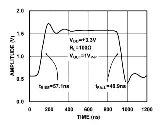
Figure9. Large-Signal Pulse Response Vs. Time(SD Channel)
