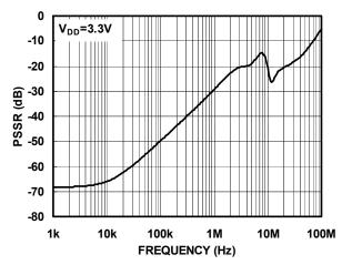
Figure7. PSRR Vs. Frequency(SD)
