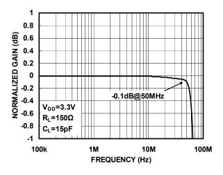
Figure2. Large-Scale Frequency Response
