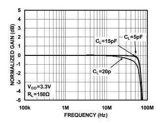
Figure4. Gain Vs. Frequency With CLOAD(FHD Channel)
