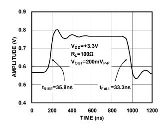
Figure10. Small-Signal Pulse Response Vs. Time(SD Channel)
