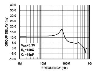
Figure6. Group Delay vs Frequency(FHD Channel)
