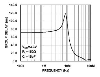
Figure5. Group Delay vs Frequency(SD Channel)
